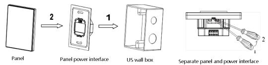
**Installation:** Hold the edge of the panel (shown as above grey area), insert the power interface module vertically. Do not push the panel too hard.
